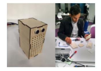
**Figure 2.** Completed fabrication of radio, with distance sensors concealed as 'eyes' (left), assembling fabricated parts together to conceal Arduino board (right).
