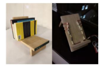
**Figure 1.** Top view of bookshelf (left), wiring and circuit view of bookshelf using conductive tape and alligator clips to connect to an Arduino (right).
